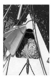
A retractable pole is employed for the asymmetric spinnaker - it was adopted from the 780 system which Darren Schofield and Steve Kiely devised and is definitely the way of the future. Intrinsic to the overall success is the kite cut by sailmaker Chris Cairns, which has heavy shoulders that float over the centreline. This allows deeper downwind angles to be attained.
