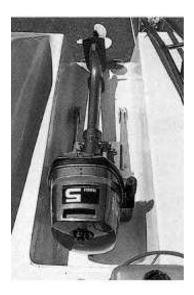
With the tiller extending further into the cockpit, the theory is that the helmsman won't go back there. In practice this has been disproved - in fact, we were all crammed aft on that high speed spinnaker reach and then the well and fuel tank get in the way. Furthermore, full mobility of the rudder is prevented when the engine is down.
